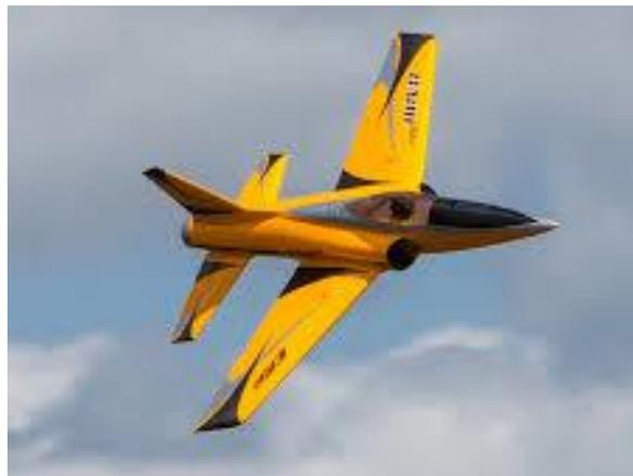
The Habu 32X has a fiberglass fuse and built-up wings, but the steady march of more and more foamy aircraft to the market is unceasing.
