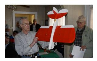
George Jones was showing the 60" GlassAir that he purchased at a swap meet. This plane appears to be larger than 60", it weighs 7.5 lbs. and is powered with an OS 91 4-stroke. The GlassAir is a model of the full size experimental aircraft. George is using a 16 x 6 prop. See photos at the top.
