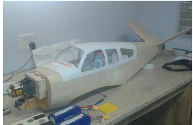
George Jones brought a newly acquired L-19 Bird Dog and won the Model of the Month. The fuse is painted fiberglass and the wings are built up wood. It is powered with an Enya 90 4-stroke. George said it has the tail off a Cessna 195 and the wings from the Cessna 170B. The plane had its maiden flight prior to the meeting, but I heard that Georg crashed it sometime this month. I'm not sure how bad it is. This photo makes the aircraft look really large, but I think the wingspan is around 95"
