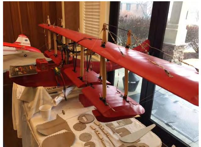
We think the motors need to be moved forward in the wing about 4+ inches, but this will require propshaft extensions and a carrier bearing. A challenge indeed.
