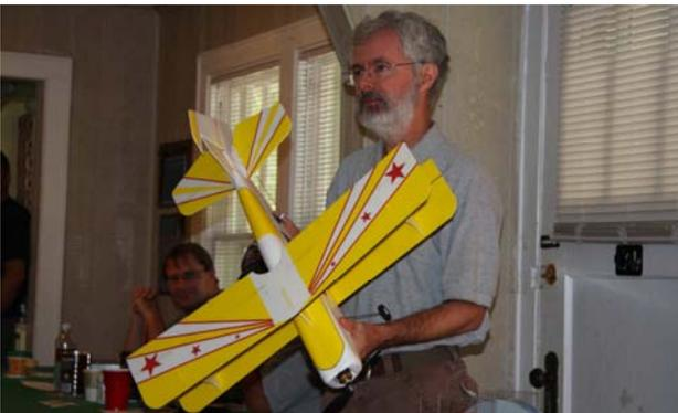
Nate Ericson was showing the scratch built "Nate's Gnat" aircraft that he built for the building contest last winter. The "Gnat" features a Turnigy ESC, a Castle Rx, and Trexler wheels. It flies on a 2S 400 mah battery, and weighs 5.5 oz's.
