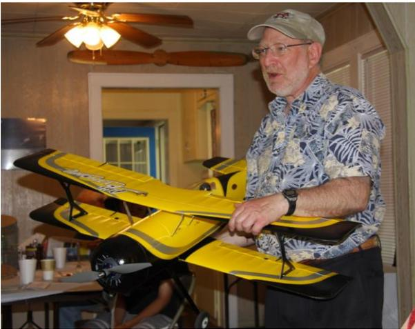
The other photo is of the 56" Maxford Globe Swift being shown by Bill Elkins. The "Swift" has flaps retracts and optional lighted instrument panel, and fly's on a 3S 3200 mah battery.
