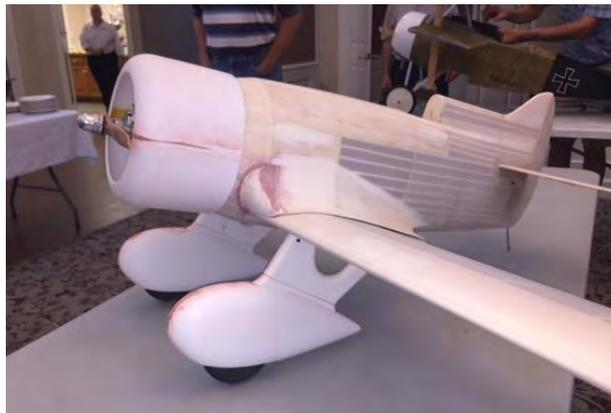
The Gee Bee is an Adrian Page kit. Ed said the landing gear fairings took as long to make as the rest of the kit. It is covered with Solar-Tex iron on fabric and powered with a Saito 56.
