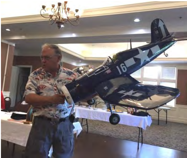
John Lagesse brought his 70" Phoenix Corsair to show. This aircraft is made in Vietnam and comes with air-retracts. John installed a Rimfire 120 and a 80 amp ESC. Theplane weighs about 12 lbs. and John flies it with a 6S Lipo.
