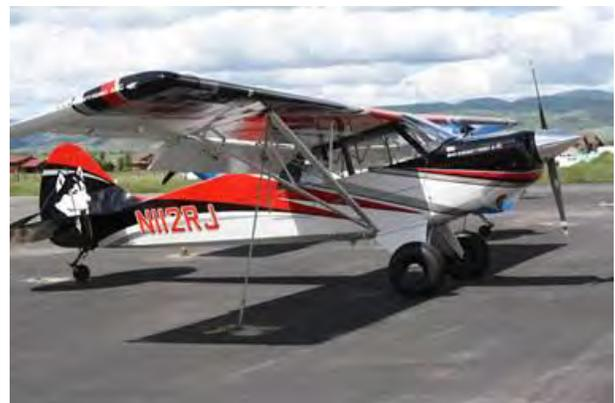
This one looked different and it's special - worlds first Tri-Fuel CNG (Compressed Natural Gas) and Low Lead Aircraft - note the unique canister on the landing gear. The belly tank was not there.
