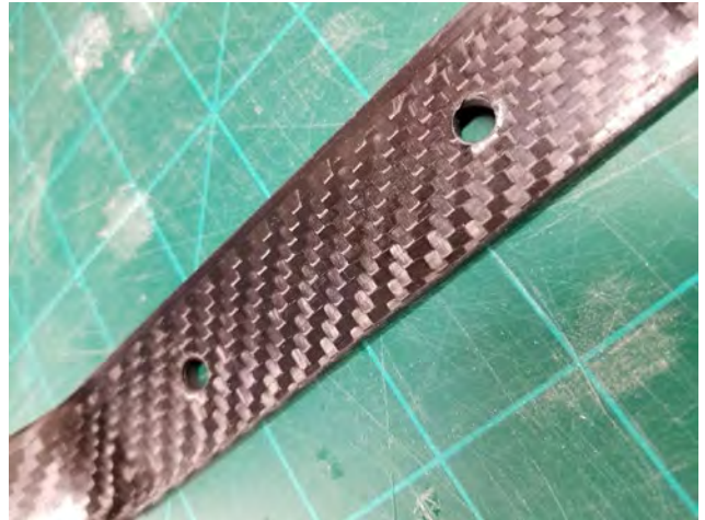
Minimal splintering with sharp drill bit and tape
