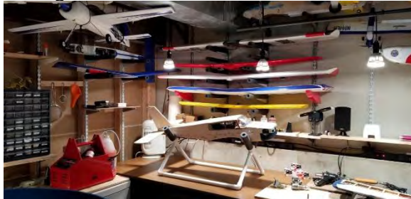
Glen's shop; note LED lights and fuselage cradle.
