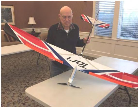
Glen Minor was showing his 33 year old rebuilt trainer from 1984; his first RC airplane. Wow, I couldn't find you my 1<sup>st</sup>, 2<sup>nd</sup> 3<sup>rd</sup> and so on airplane. Whole airplane was recovered, and an Eflite 480 motor installed. It flies on a 3S battery with a 40 amp Esc. Glen won the MOM; model of the month.
