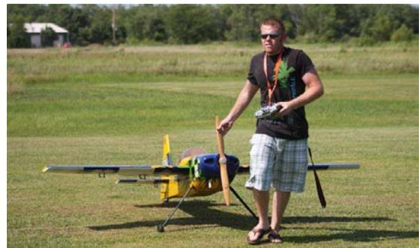
Unfortunately, Alex damaged the 101" Edge 540 Sunday when he ran out of fuel doing a 3-D maneuver about 10 feet above the ground. I believe he broke the firewall loose and cracked part of the cowl.
